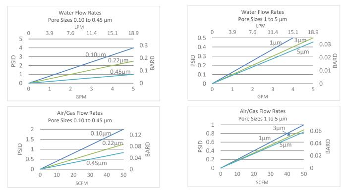
Flow rates for Cartridge filters are per 10-inch length. The test fluid is water or compressed air at ambient temperature.
