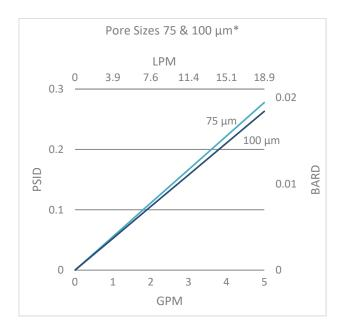
Flow rates shown are for pleated cartridges per 10-inch length. The test fluid is water at ambient temperature.
