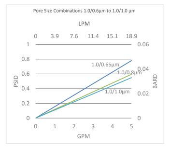
Flow rates for Cartridge filters are per 10-inch length. The test fluid is water at ambient temperature.
