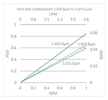
Flow rates for Capsule filters are per square foot of membrane area. The test fluid is water at ambient temperature. Flows are tested using a 2" capsule filter with ½" FNPT inlet and outlet ports. Rates will vary based on end configuration of the capsule.
