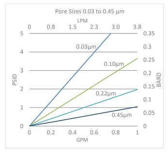
Flow rates for Capsule filters are per square foot of membrane area. The test fluid is water at ambient temperature. Flows are tested using a 2" capsule filter with %" FNPT inlet and outlet ports. Rates will vary based on end configuration of the capsule.
