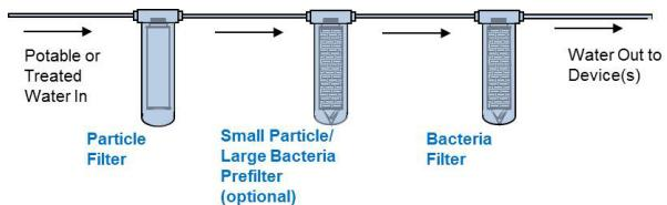
**Figure 2 - Filters in a Central Water System for a Healthcare Facility**
