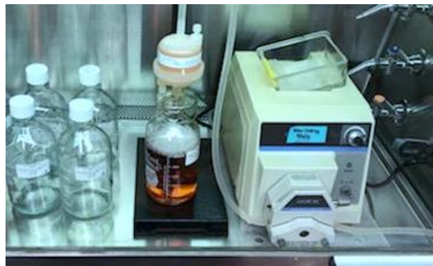
Critical Process Filtration's SPS Mini-Capsule in use for Cell Culture Media Filtration
