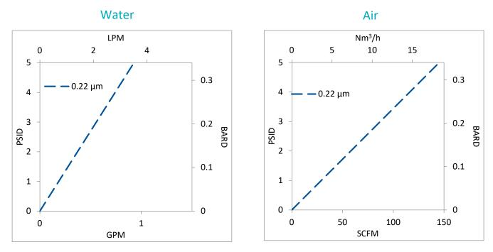
Flow Rates for PPVWB/GS Standard Capsules by Pore Size
