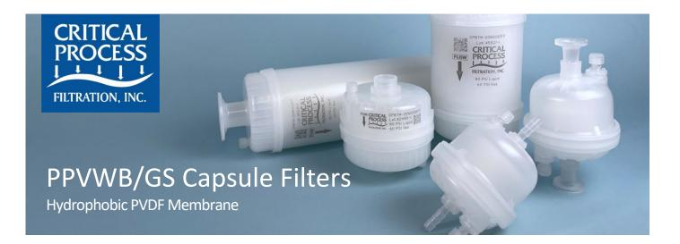
PPVWB/GS Filters consist of a single layer, hydrophobic, high capacity polyvinylidene fluoride (PVDF) membrane. Designed to be incorporated in single use systems, the PPVWB/GS is constructed with gamma stable polypropylene materials. These capsule filters come in a variety of sizes: Mini, 2, 5, 10, 20 and 30 inches. Each device is available in 0.22 microns.
