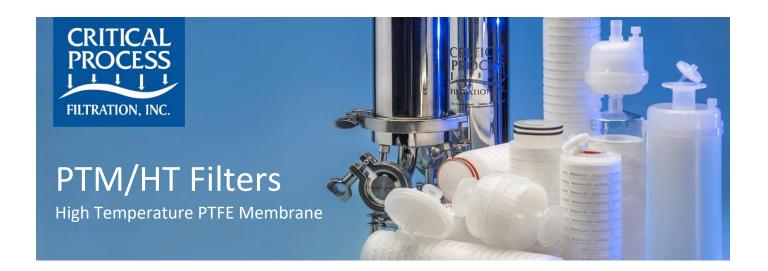
PTM/HT cartridge filters are made with Polytetrafluoroethylene (PTFE) membrane and high temperature polypropylene for cartridge hardware and membrane support. The filters are validated for sterilizing in elevated temperature gas and non-aqueous liquid applications (up to 221°F). Pore sizes range from 0.10 to 1.0  $\mu m$ .
