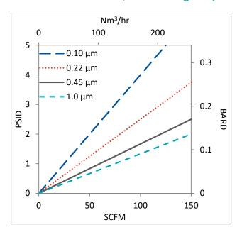
Flow rates for Cartridge filters are per 10-inch length. The test fluid is water or air at ambient temperature.
