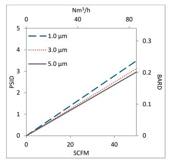
Flow rates for Capsule filters are tested using a 2" capsule filter with 1" sanitary inlet and outlet ports. The test fluid is water or compressed air at ambient temperature. Flow rates for larger capsules will scale with filtration area. Rates will vary based on end configuration of the capsule.
