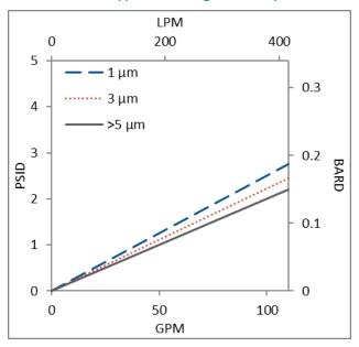
Flow rates for Cartridge filters are for a single #2 bag filter. The test fluid is water at ambient temperature. Recommended flow rate for #2 bag not to exceed 110 GPM.
