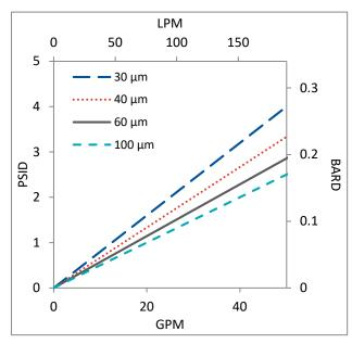
Flow rates for Cartridge filters are per 10-inch length. The test fluid is water at ambient temperature.
