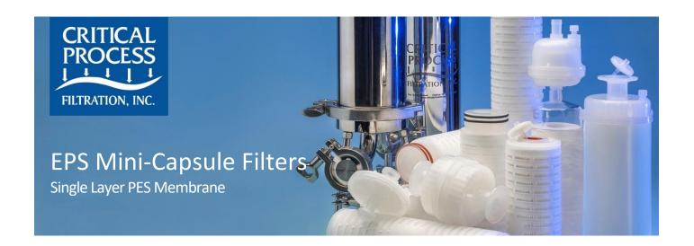
EPS Mini-Capsule filters are constructed with a single layer Polyethersulfone (PES) membrane. They are designed for the electronics industry and used for removing fine and ultrafine particles from aqueous liquids. Pore sizes range from 0.02 to 0.45  $\mu m$  and the filter devices scale from laboratory to full production using identical materials to ensure consistent results.
