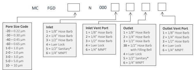
\*When choosing the Sanitary Inlet/Outlet, the Luer Lock option is required for the Vent Port
