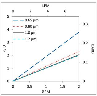
Flow rates for Mini-Capsule filters are per filter. The test fluid is water at ambient temperature. Flows are tested using a mini-capsule filter with  $\frac{1}{2}$ " Sanitary inlet and outlet ports. Rates will vary based on end configuration of the mini-capsule.
