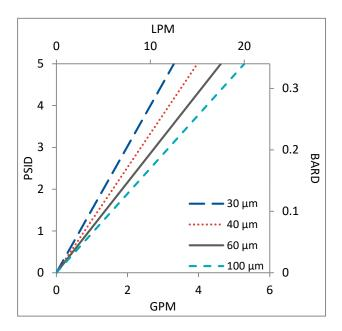
Flow rates for Mini-Capsule filters are per filter. The test fluid is water at ambient temperature. Flows are tested using a mini-capsule filter with ½" Sanitary inlet and outlet ports. Rates will vary based on end configuration of the mini-capsule.
