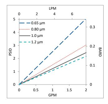
Flow rates for Mini-Capsule filters are per filter. The test fluid is water at ambient temperature. Flows are tested using a mini-capsule filter with  $\frac{1}{2}$ " Sanitary inlet and outlet ports. Rates will vary based on end configuration of the mini-capsule.
