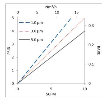
Flow rates for Mini-Capsule filters are per filter. The test fluid is compressed air at ambient temperature. Flows are tested using a mini-capsule filter with %" Sanitary inlet and outlet ports. Rates will vary based on end configuration of the mini-capsule.
