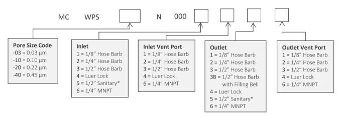
\*When choosing the Sanitary Inlet/Outlet, the Luer Lock option is required for the Vent Port
