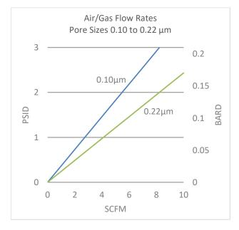
Flow rates for Capsule filters are per square foot of membrane area. The test fluid is water or compressed air at ambient temperature. Flows are tested using a 2" capsule filter with ½" FNPT inlet and outlet ports. Rates will vary based on end configuration of the capsule.
