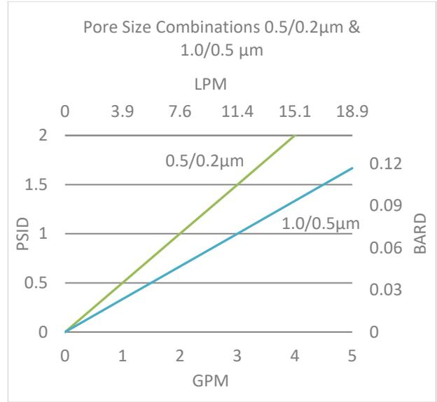
Flow rates for Cartridge filters are per 10-inch length. The test fluid is water at ambient temperature.
