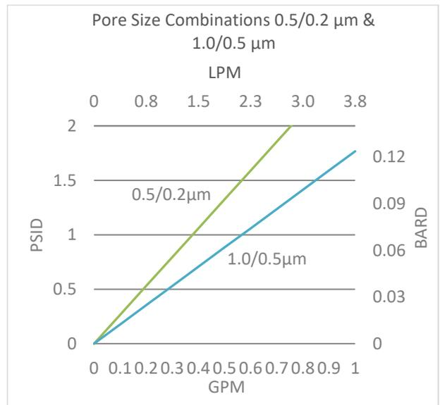
Flow rates for Capsule filters are per square foot of membrane area. The test fluid is water at ambient temperature. Flows are tested using a 2" capsule filter with 1/2" FNPT inlet and outlet ports. Rates will vary based on end configuration of the capsule.
