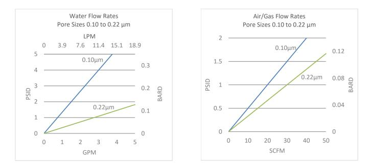
Flow rates for Cartridge filters are per 10-inch length. The test fluid is water or compressed air at ambient temperature.
