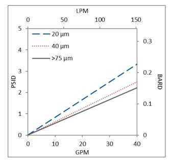
Flow rates shown are for pleated cartridges per 10-inch length. The test fluid is water at ambient temperature.
