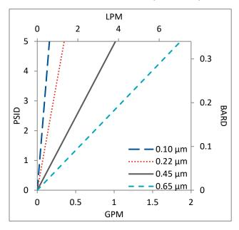
Flow rates for Micro Capsule filters are per filter. The test fluid is water at ambient temperature. Flows are tested using a Micro capsule filter with  $\chi''$  Sanitary inlet and outlet ports. Rates will vary based on end configuration of the Micro capsule.
