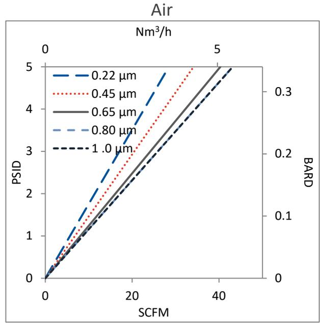
Flow rates for Micro Capsule filters are per filter. The test fluid is water at ambient temperature. Flows are tested using a Micro capsule filter with 1/2" Sanitary inlet and outlet ports. Rates will vary based on end configuration of the Micro capsule.
