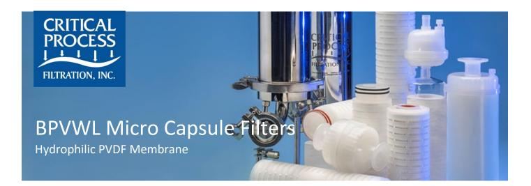
BPVWL Micro Capsule filters consist of a single layer, hydrophilic, high capacity polyvinylidene fluoride (PVDF) membrane. These filters are used for bioburden control and clarification/prefiltration in aqueous liquids. Pore sizes range from 0.22 to 1.0  $\mu$ m, and are available pre-sterilized.
