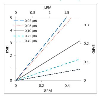
Flow rates for Micro Capsule filters are per filter. The test fluid is water at ambient temperature. Flows are tested using a Micro capsule filter with \%" Sanitary inlet and outlet ports. Rates will vary based on end configuration of the Micro capsule.
