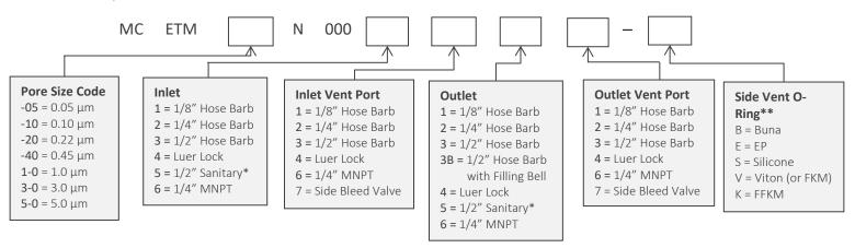
\*When choosing the Sanitary Inlet/Outlet, the Luer Lock or bleed valve option is required for the Vent Port
