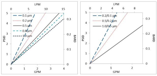
Flow rates for Micro Capsule filters are per filter. The test fluid is water at ambient temperature. Flows are tested using a Micro capsule filter with ½" Sanitary inlet and outlet ports. Rates will vary based on end configuration of the Micro capsule.
