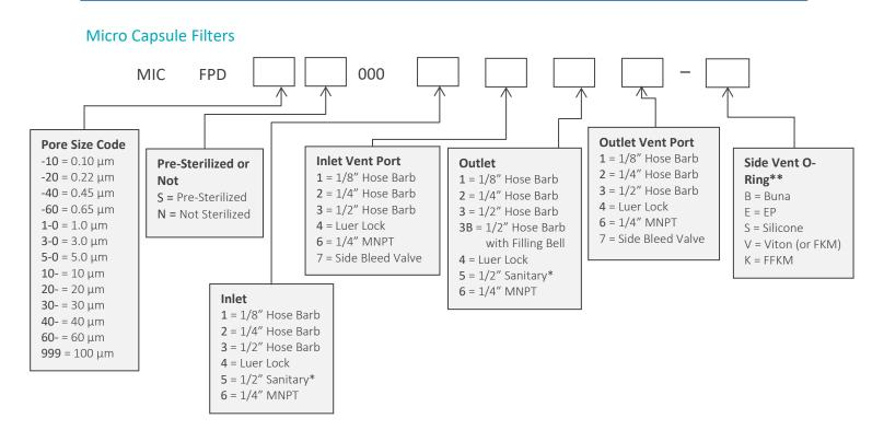
\*When choosing the Sanitary Inlet/Outlet, the Luer Lock or bleed valve option is required for the Vent Port
