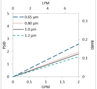
Flow rates for Micro Capsule filters are per filter. The test fluid is water at ambient temperature. Flows are tested using a Micro capsule filter with 1/2" Sanitary inlet and outlet ports. Rates will vary based on end configuration of the Micro capsule.
