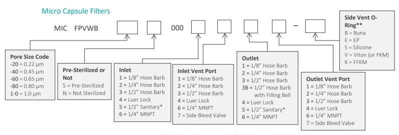
$\hbox{$^*$When choosing the Sanitary Inlet/Outlet, the Luer Lock or bleed valve option is required for the Vent Port}\\$
