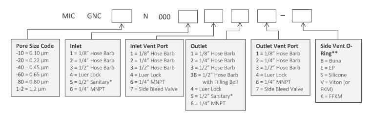
\*When choosing the Sanitary Inlet/Outlet, the Luer Lock or bleed valve option is required for the Vent Port
