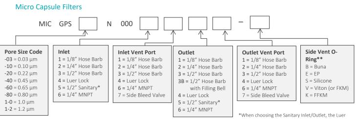
\*When choosing the Sanitary Inlet/Outlet, the Luer Lock or bleed valve option is required for the Vent Port \*\* O-Ring is only available on Bleed Valve
