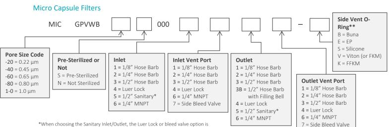
\*When choosing the Sanitary Inlet/Outlet, the Luer Lock or bleed valve option is required for the Vent Port
