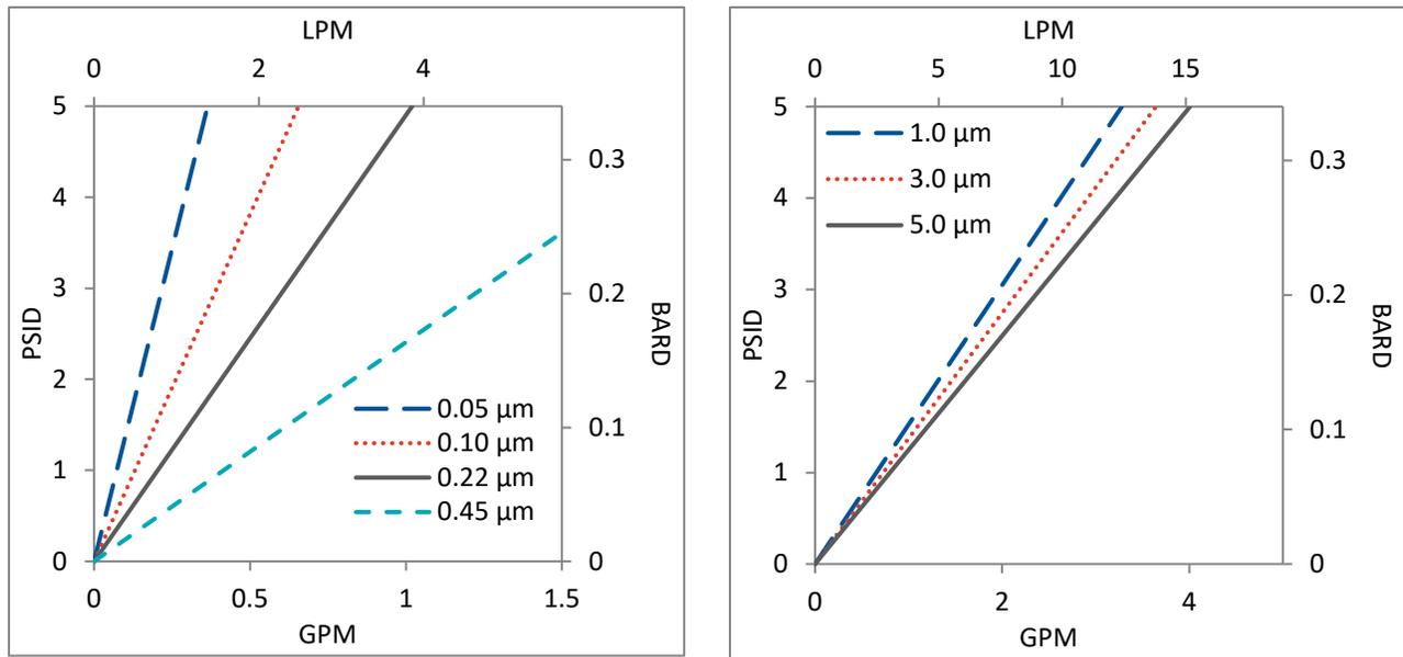
Flow rates for Micro Capsule filters are per filter. The test fluid is water at ambient temperature. Flows are tested using a Micro capsule filter with 1/2" Sanitary inlet and outlet ports. Rates will vary based on end configuration of the Micro capsule.
