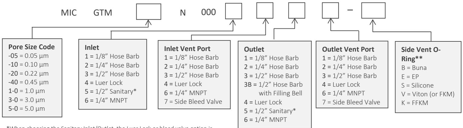
\*When choosing the Sanitary Inlet/Outlet, the Luer Lock or bleed valve option is required for the Vent Port
