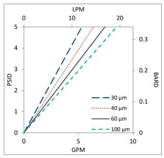
Flow rates for Micro Capsule filters are per filter. The test fluid is water at ambient temperature. Flows are tested using a Micro capsule filter with  $\frac{1}{2}$ " Sanitary inlet and outlet ports. Rates will vary based on end configuration of the Micro capsule.
