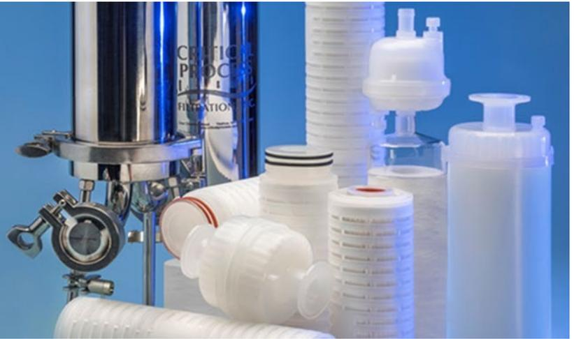
PGD cartridge and capsule filters are constructed with fiberglass depth media for clarification and prefiltration of aqueous liquids. Pore sizes range from 0.22 to 5.0  $\mu\text{m}$  and filter sizes scale from laboratory to full production using identical materials to ensure consistent results.
