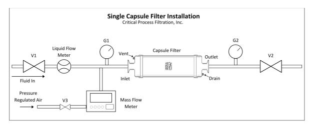
Capsule filters are self-contained, disposable units that do not require any additional housings. The units may be installed and operated using the steps below.
