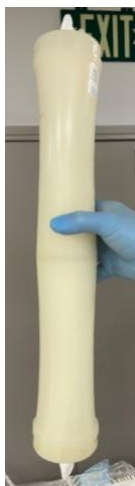
Figure 1: Capsule Shell Collapse due to Vacuum during Cooling
